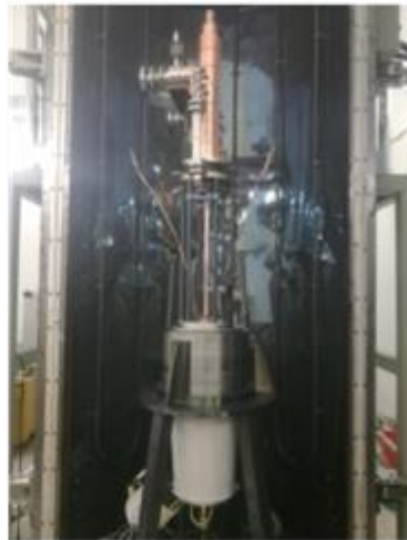
BVEI X-band 50 MW 57% COM Prototype
