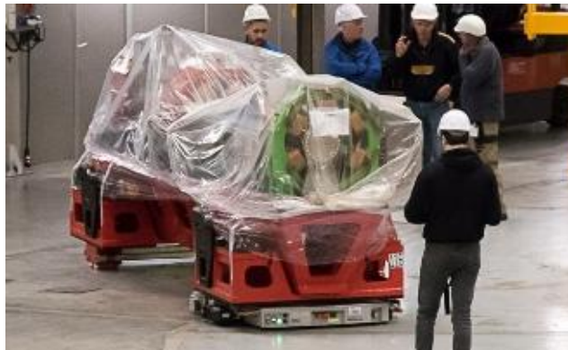
Movers similar to those used for EBS will be used to move equipment inside the tunnel (No crane).
