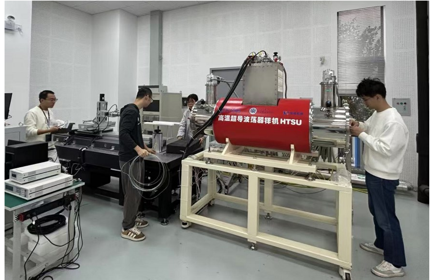
Full assembly of HTSU12 and the associated magnetic field measurement system
