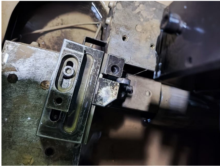
EDM to cut the bulk
