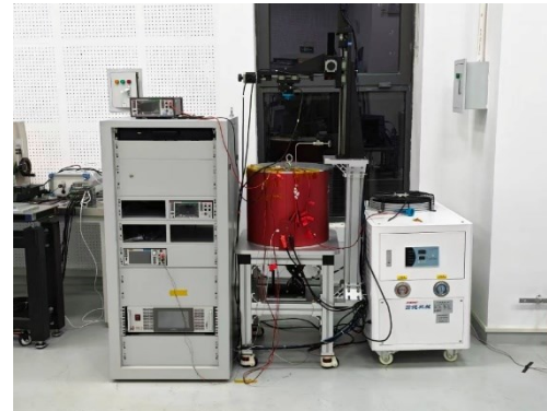
Vertical field measurement system equipped with 0.3 T solenoid and 77 K
