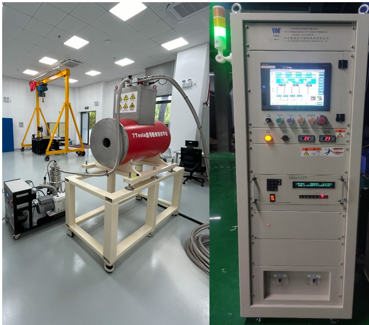
On-site test of the 7 T solenoid
