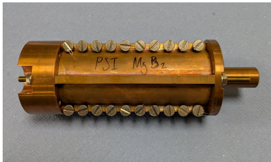
\text{MgB}_2 short model: \lambda_u = 16 mm, g = 4 mm
