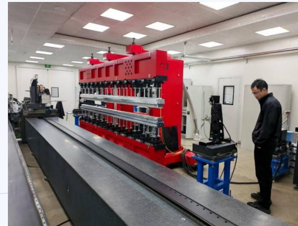
IVU21a shimming and test
