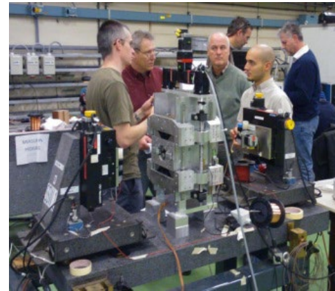
Left: Longitudinal gradient dipole magnet for the CLIC DR (CIEMAT)
