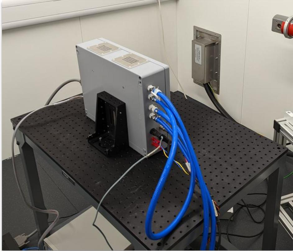
*HEXITEC<sub>MHz</sub> test enclosure (exterior)*
