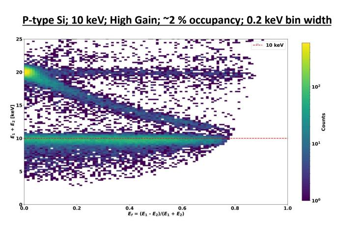
The distribution of energies in two-pixel charge sharing events using a 10 keV beam energy at an occupancy of ~2% - 0.2 keV bin width
