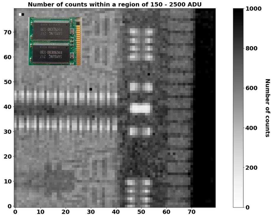
*X-Ray transmission measurements of a DDR Ram Card using a HEXITEC<sub>MHz</sub> HF-CZT sensor*
