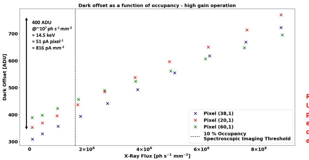
HF-CZT detector @ -1000 V @ 20 keV: Variation of dark offset with X-Ray flux
