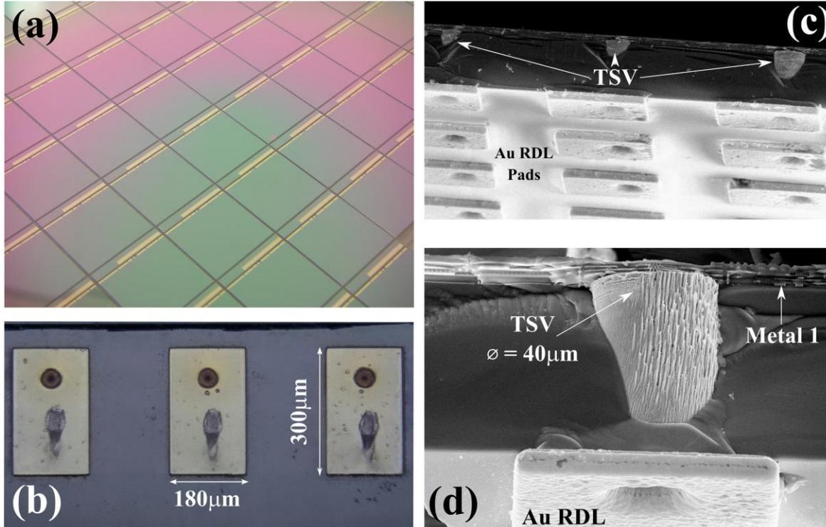
(a) I/O pads on reverse of the 200 mm HEXITEC<sub>4S</sub> wafer post-TSV-last processing. (b) RDL pads dimensions on ASIC's reverse. (c) SEM micrograph of exposed TSVs in cleaved test chip. (d) SEM micrograph showing contact between TSV and ASIC's bottom metal layer
