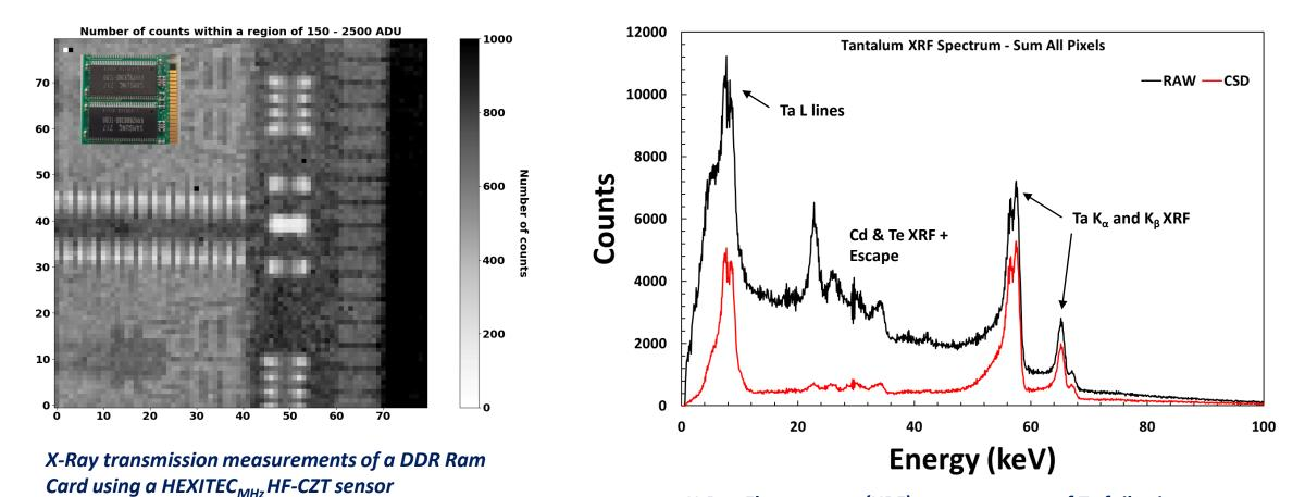
X-Ray Fluorescence (XRF) measurements of Ta foil using a  $HEXITEC_{MHz}$  HF-CZT sensor in medium-gain mode
