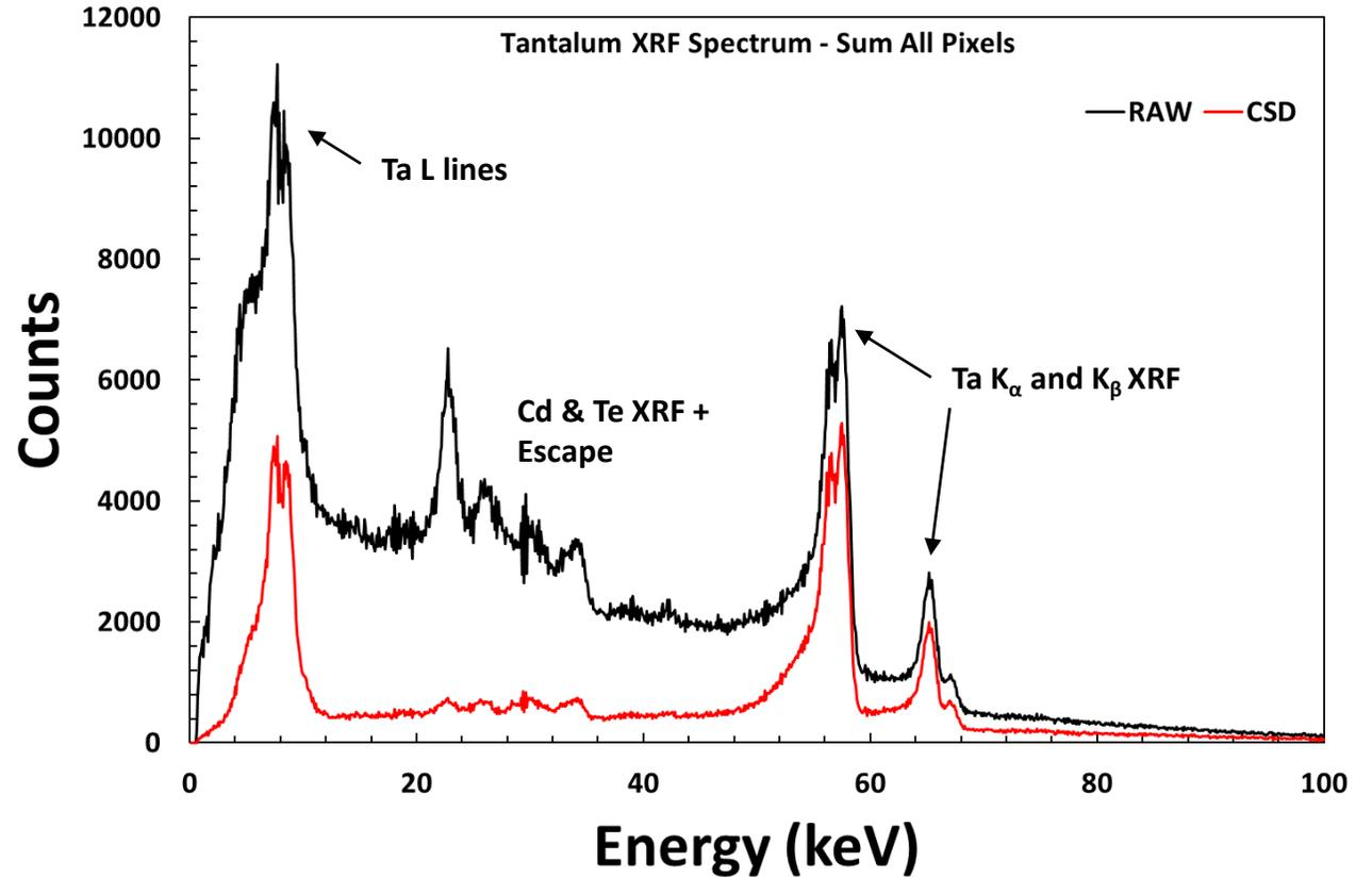
*X-Ray Fluorescence (XRF) measurements of Ta foil using a HEXITEC<sub>MHz</sub> HF-CZT sensor in medium-gain mode*
