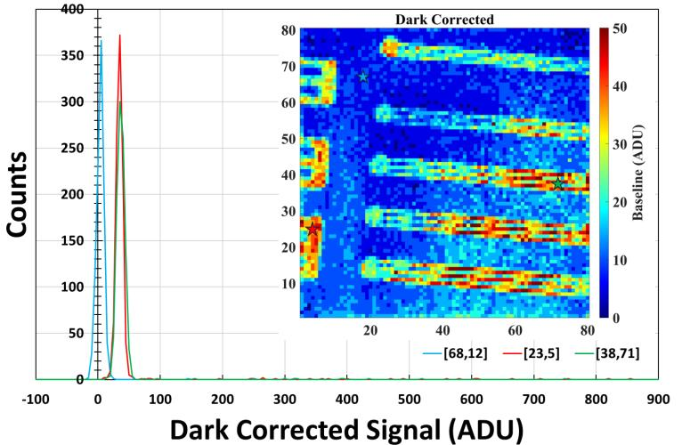
Histograms of signals measured in three pixels from different areas in the irradiation showing different offsets. (Inset) A map of dark-offset
