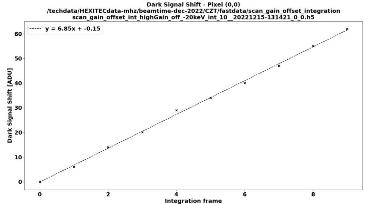
Linear-fit calculation to a plot of dark offset vs frames following reset
