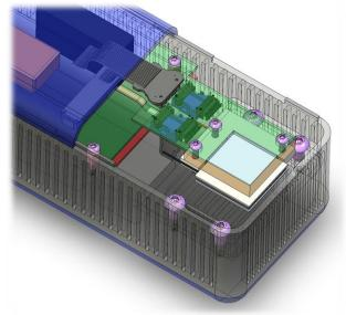
Possible designs for HEXITEC<sub>MHz</sub> detector system
