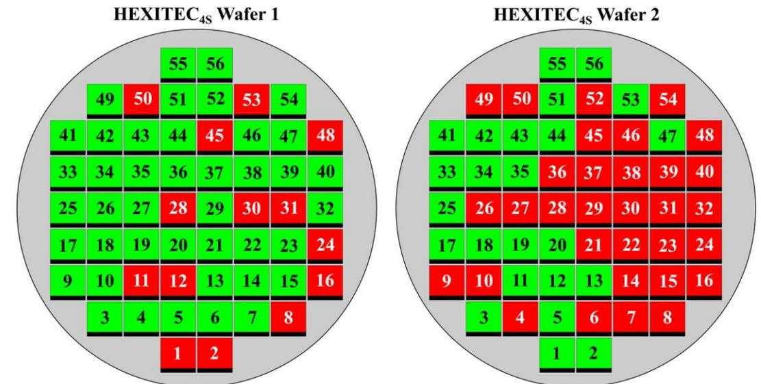
Wafer maps showing results of probe testing.
