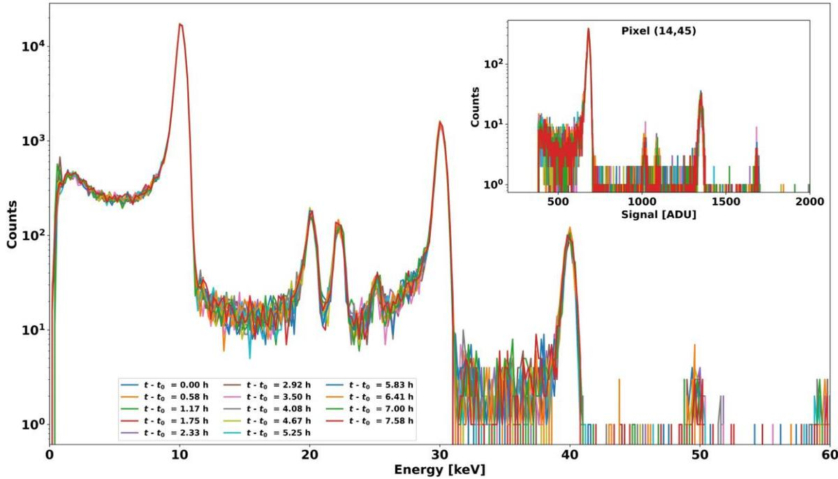
Evolution of high-gain calibrated global CSD spectra during exposure @ 10 keV for ~8 h – 0.2 keV bin width. Inset plot shows uncalibrated CSD spectra for pixel (14,45) – 1 ADU bin width
