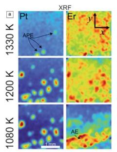
Figure 7. (a) Pt and Er XRF intensity maps as a function of temperature during the solidification of an Al-23Pt-20Er alloy at 0.1  $\rm Ks^{-1}.$
