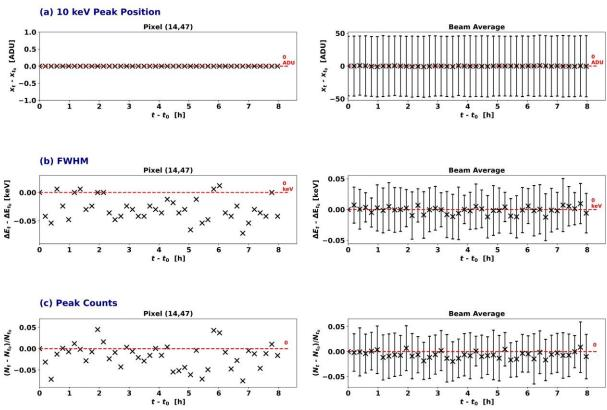
Change in performance of p-type  $\text{HEXITEC}_{\text{MHz}}$  device during exposure @ 10 keV for ~8 h. Plots show fluctuation in peak position (a), change in FWHM (b), and fractional change in peak counts (c) of 10 keV photo peak. Peak counts comprise events within the FWHM of peak, and error bars given by standard deviation across beam region
