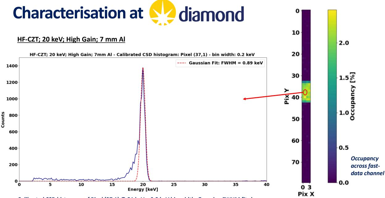
Calibrated CSD histogram of Pixel (37,1) @ 21 keV – 0.2 keV bin width. Gaussian FWHM fit shown
