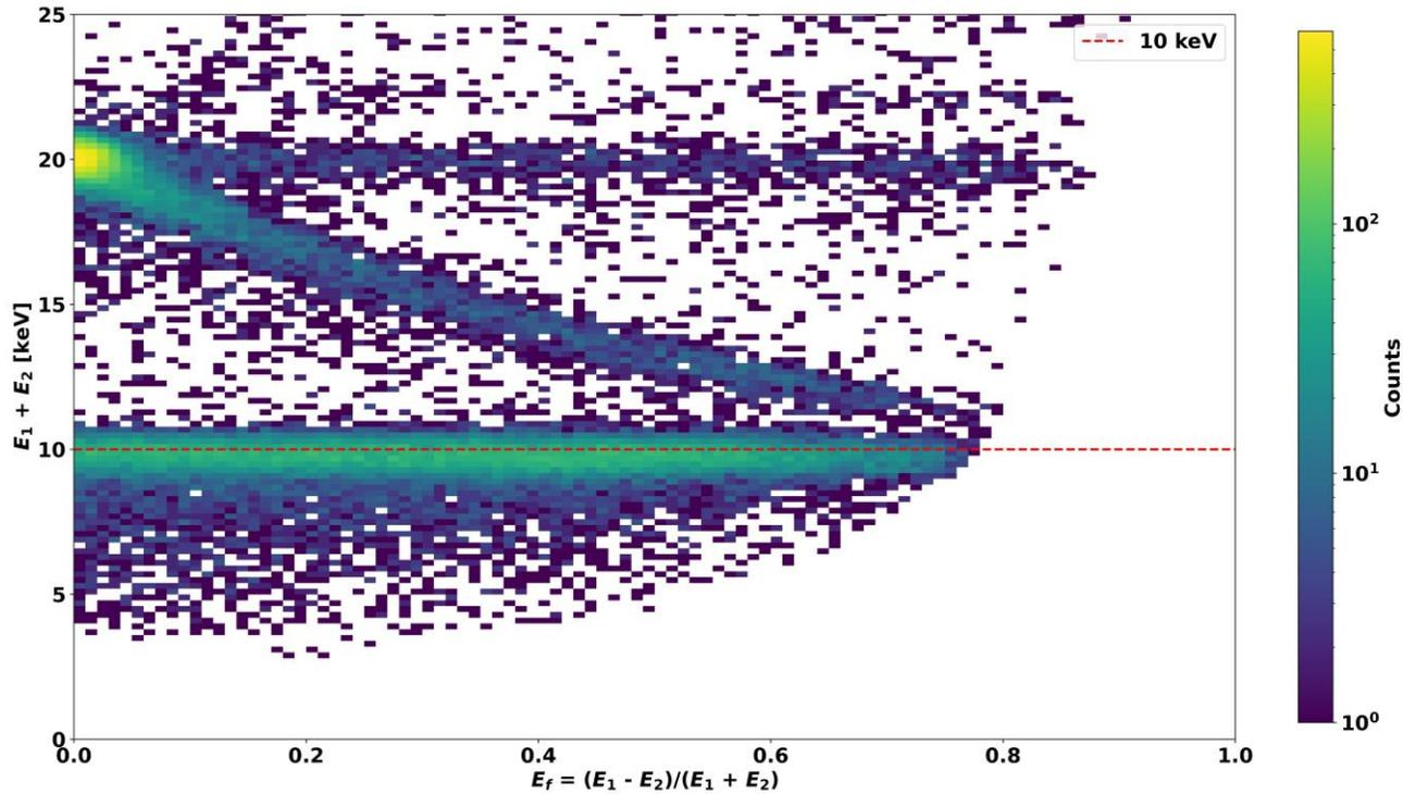
*The distribution of energies in two-pixel charge sharing events using a 10 keV beam energy at an occupancy of ~2% - 0.2 keV bin width*
