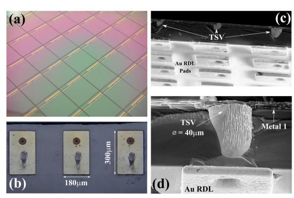
(a) I/O pads on reverse of the 200 mm HEXITEC4S wafer post-TSV-last processing. (b) RDL pads dimensions on ASIC's reverse. (c) SEM micrograph of exposed TSVs in cleaved test chip. (d) SEM micrograph showing contact between TSV and ASIC's bottom metal layer
