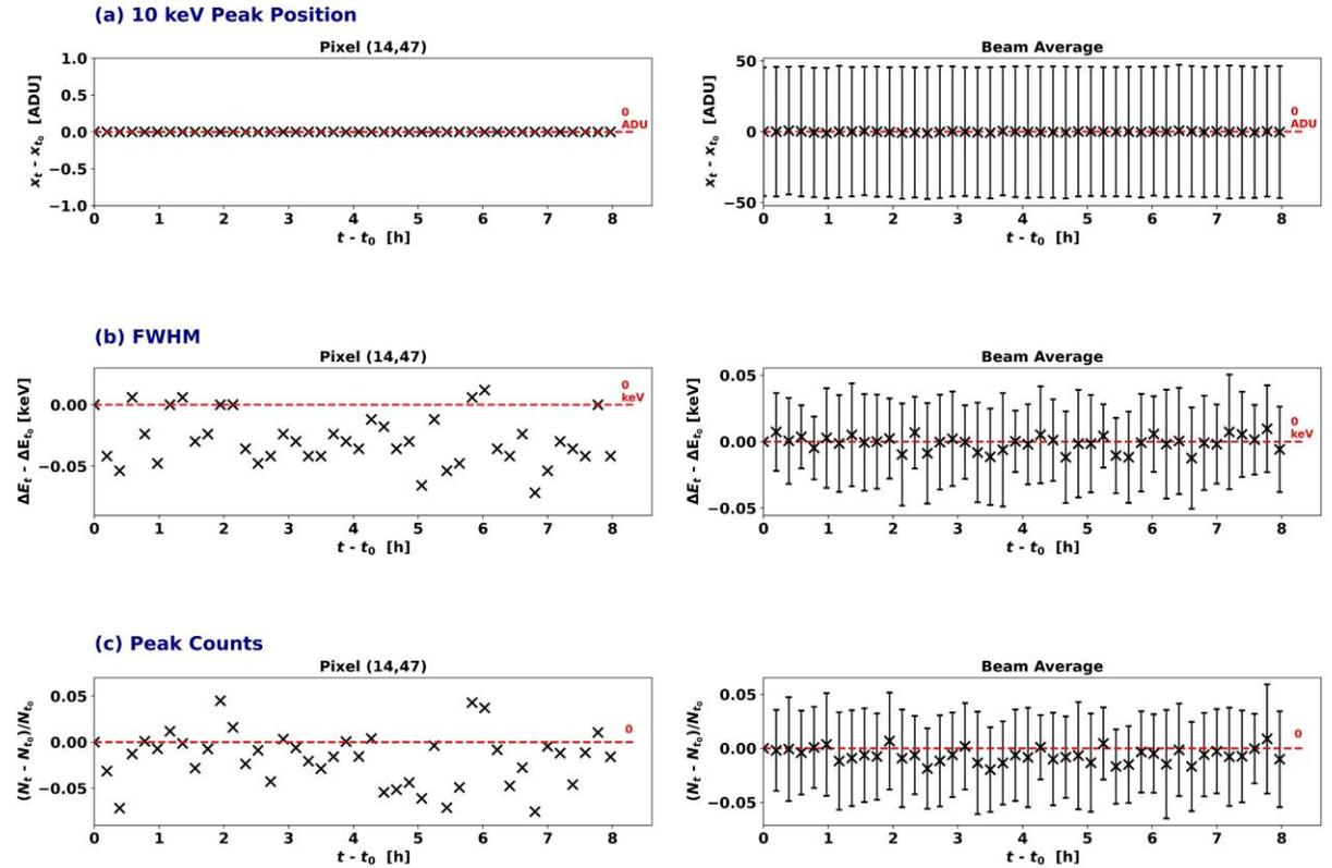
Change in performance of p-type HEXITEC<sub>MHz</sub> device during exposure @ 10 keV for ~8 h. Plots show fluctuation in peak position (a), change in FWHM (b), and fractional change in peak counts (c) of 10 keV photo peak. Peak counts comprise events within the FWHM of peak, and error bars given by standard deviation across beam region
