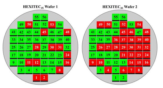
Wafer maps showing results of probe testing. Green – functioning; Red – non-functioning
