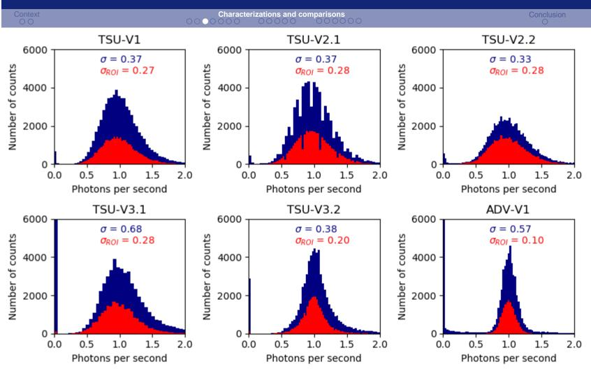
$\Rightarrow$  The most homogenous sensors are ADV-V1 and TSU-V3.2 (ROI measurements)
