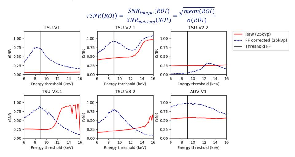
$\Rightarrow$  The FF correction effectively improves the rSNR for all detectors (except TSU-V2.2)
