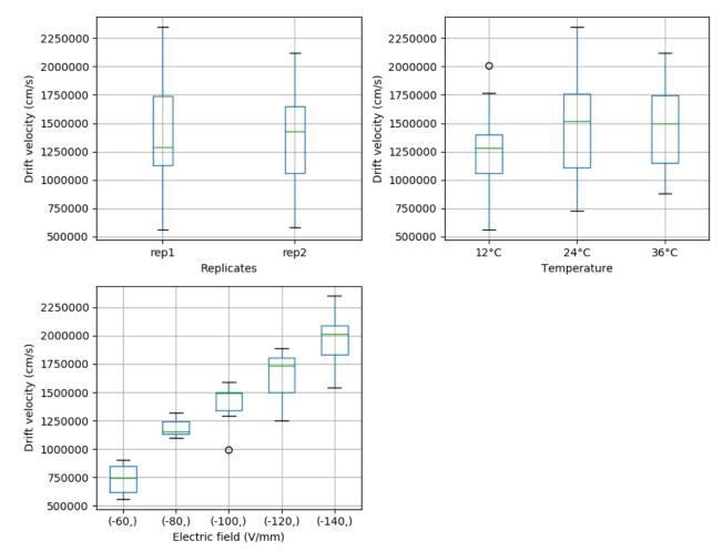
$\Rightarrow$  The drifts velocity depends only on electric field (saturation not reached)
