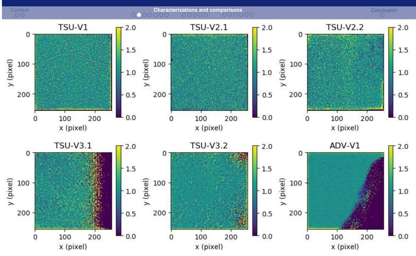
$\Rightarrow$  Bonding and breakage issues with the most recent detectors
