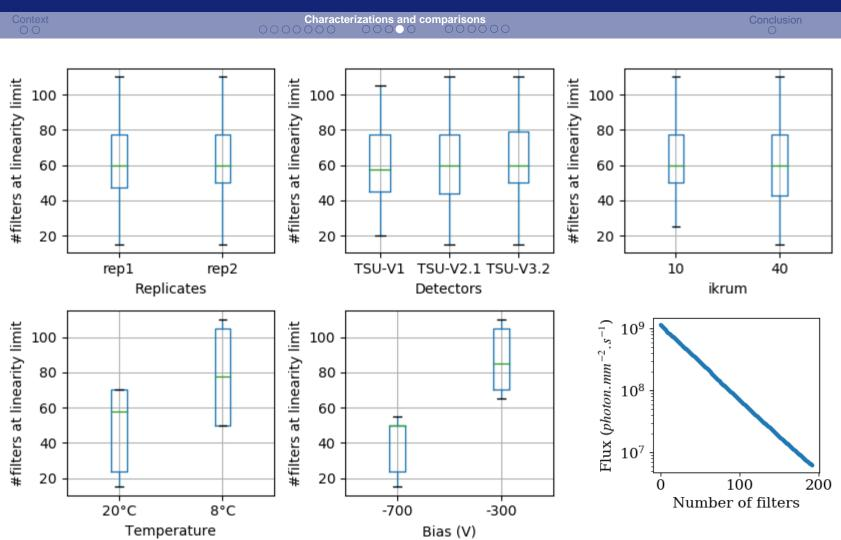
$\Rightarrow$  The linearity limit increases with both the temperature and the bias.
