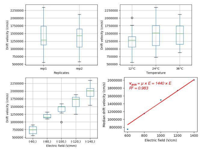
$\Rightarrow$  The drifts velocity depends only on electric field (saturation not reached)
