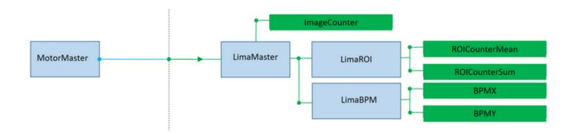
AcquisitionChain reflects the devices triggering hierarchy
