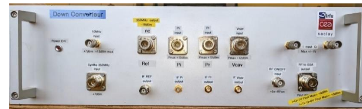
RF interface (frequency translation to 10 MHz)
