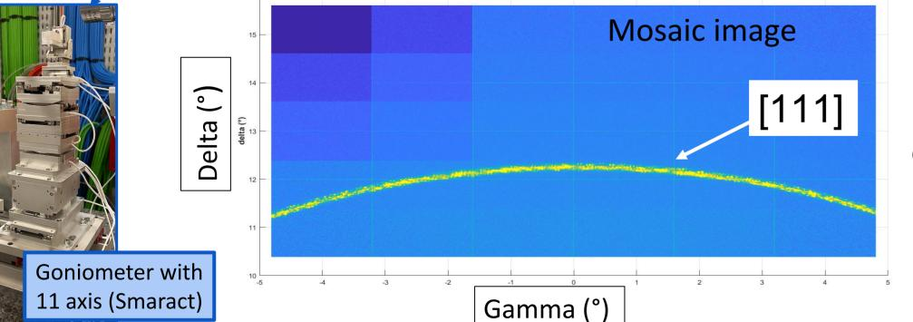
diffraction Powder X-ray measurement @ 14 keV with unfocused beam of a Si calibration sample.
