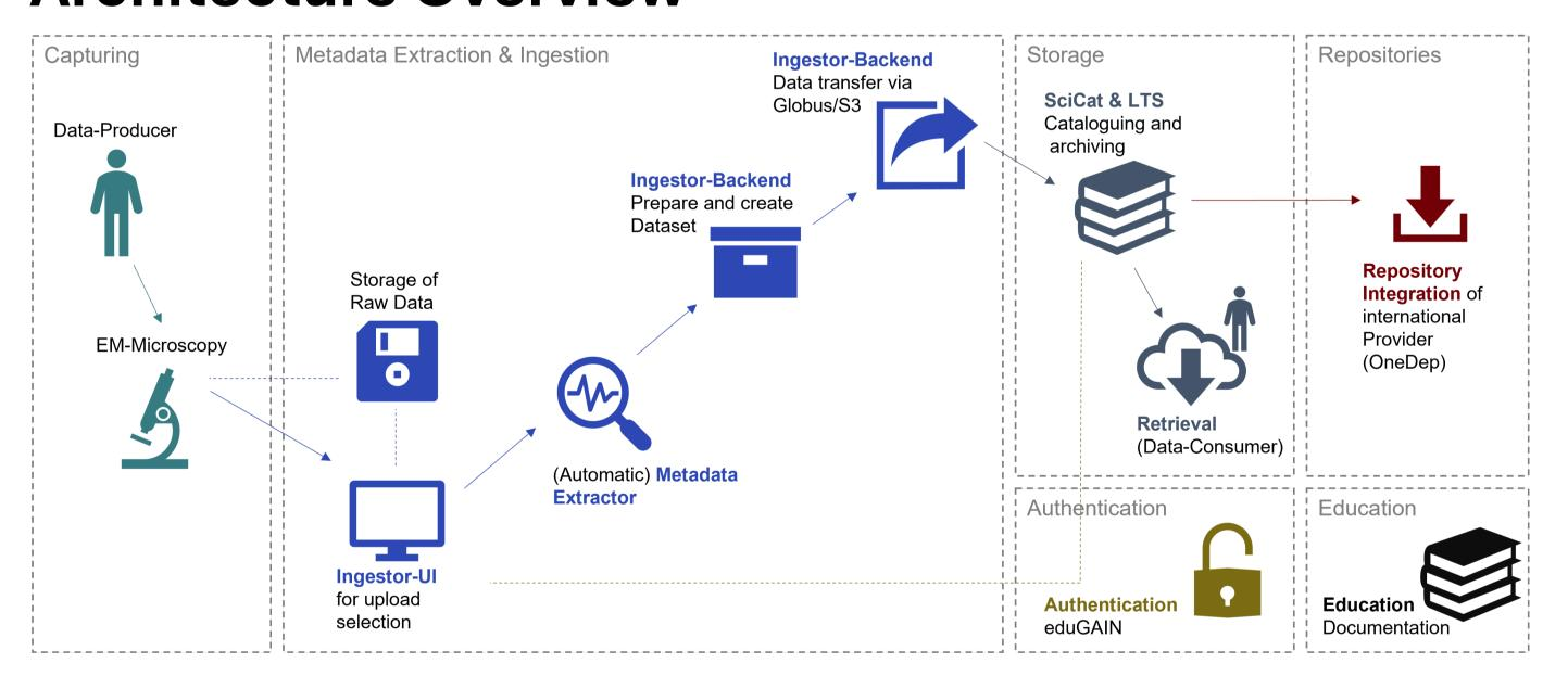
The OpenEM ecosystem is built on a microservice architecture. Users interact with the central SciCat Data Catalog at PSI, which provides the user interface, backend API, storage for metadata in MongoDB, and integration with external services. Authentication is supplied by the eduGAIN federation, allowing users from most academic institutes to access the service.
