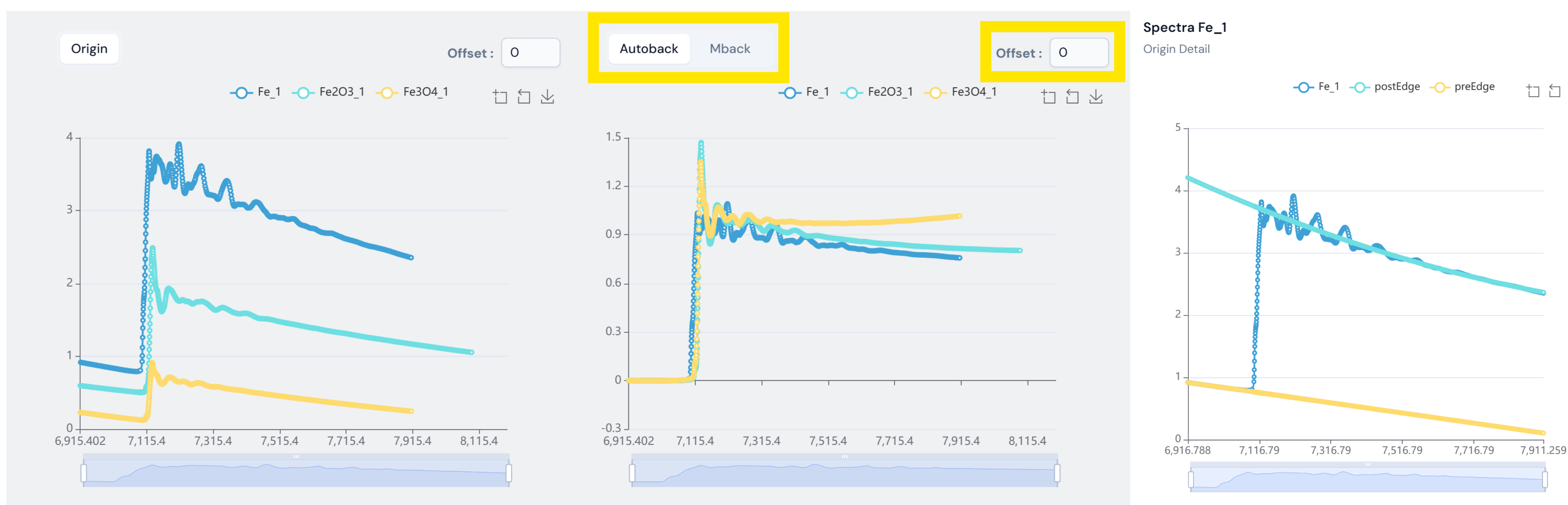
Figure 7: Absorption spectra visualization function display diagram. Users can select multiple absorption spectra for comparison at the same time, and can choose Autoback or Mback method to normalize the absorption spectra. We provide the display of pre_edge and post_edge functions, as well as the offset function.
