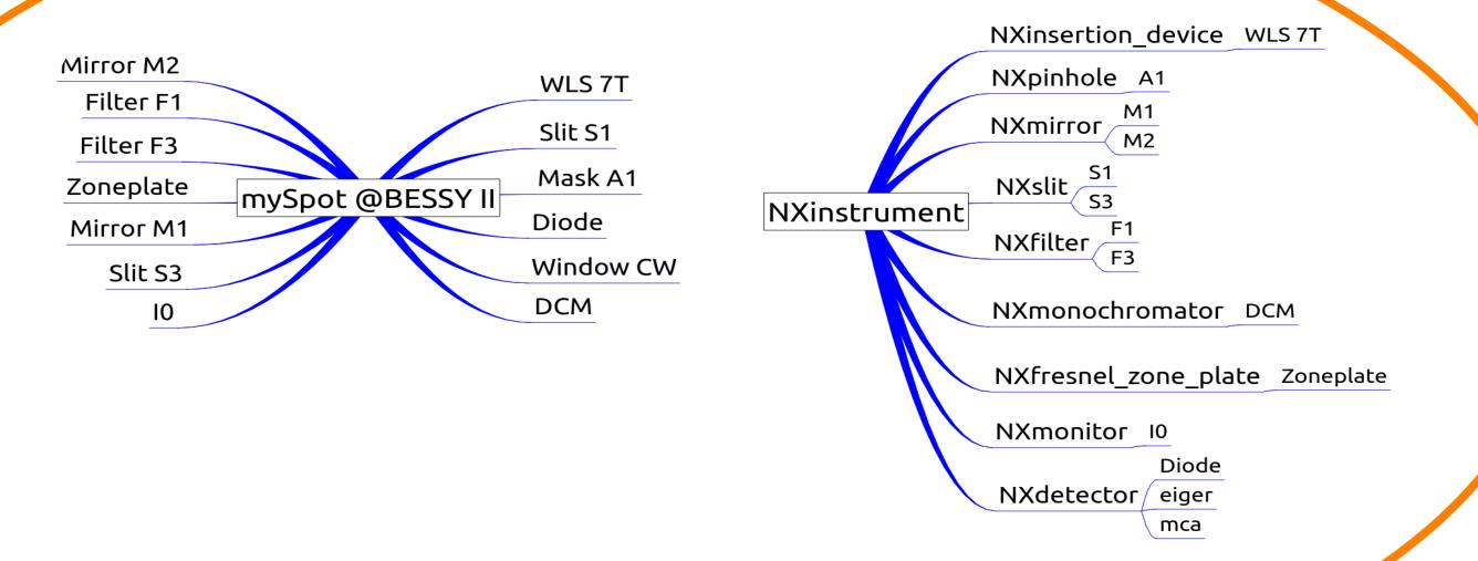
Figure 3: Mapping of mySpot beamline instruments to NeXus base class
