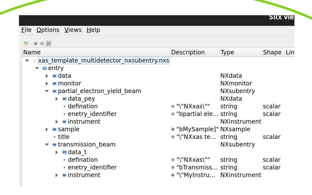
Figure 4: Example structure of NeXus hdf5 file incorporating XAS measurement in multi-mode
