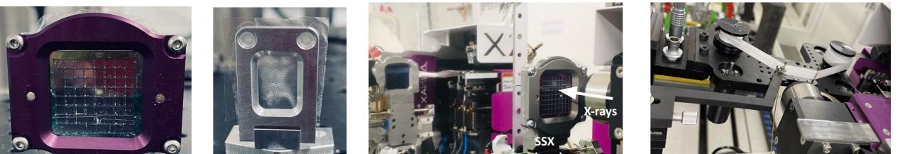
that eases data collection also for non expert users. Fixed target acquisition is either performed on foils or Silicon chips by continuous scanning along an S-shape trajectory. Silicon chips are automatically aligned prior the data acquisition.
